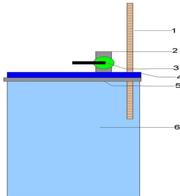
1. Thermometer. 2. Valve tube. 3. The valve. 4. The cover. 5. The locking belt. 6. The tank.
